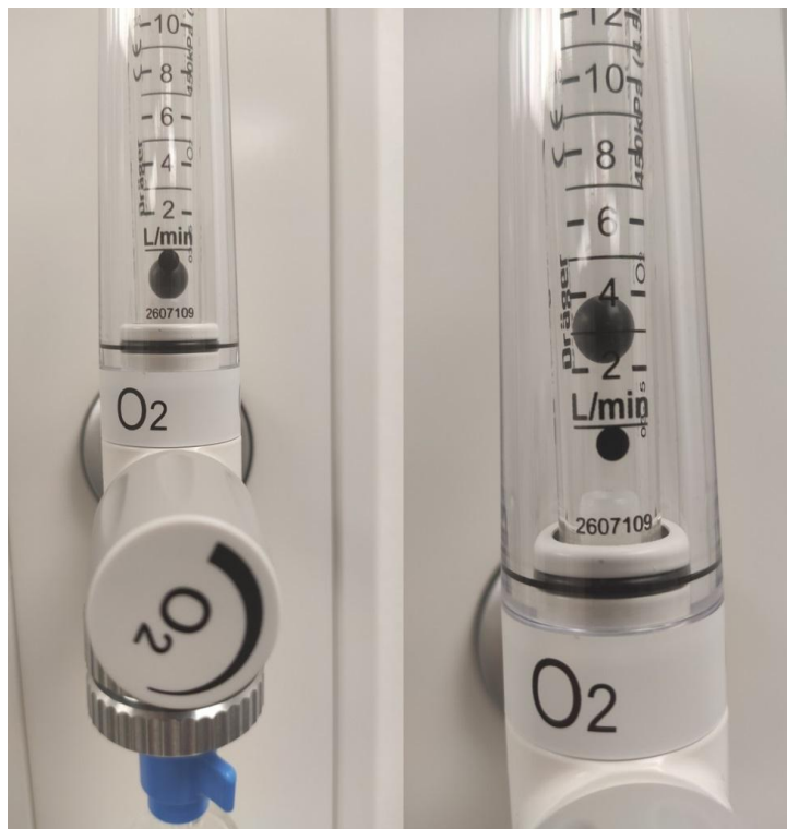
Figure 4: Correct reading of the floating ball (here on the “north pole”) on a tube flow meter (the flow rate is set to 4 L O 2 /min, as shown in the right image)
